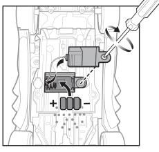
Batteries are to be inserted with the correct polarity. Exhausted batteries are to be removed from the product.
